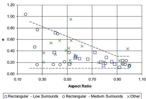
Figure 1. Eccentricity factor based on peak torsional moment and the corresponding along wind force for the three building groups.
