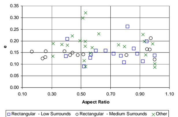
Figure 2. Eccentricity factor based on peak torsional moment and the maximum peak along wind force for the three building groups.
