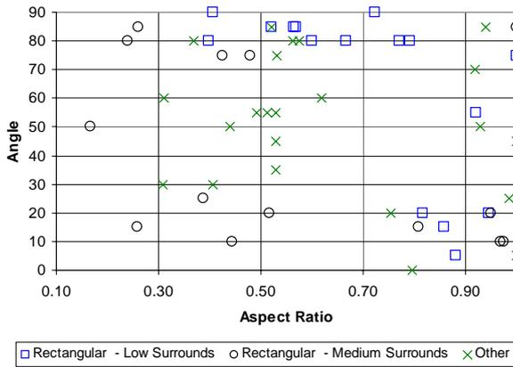
Figure 4. Angle between the wind direction inducing the largest torsional moment and direction normal to the widest face.
