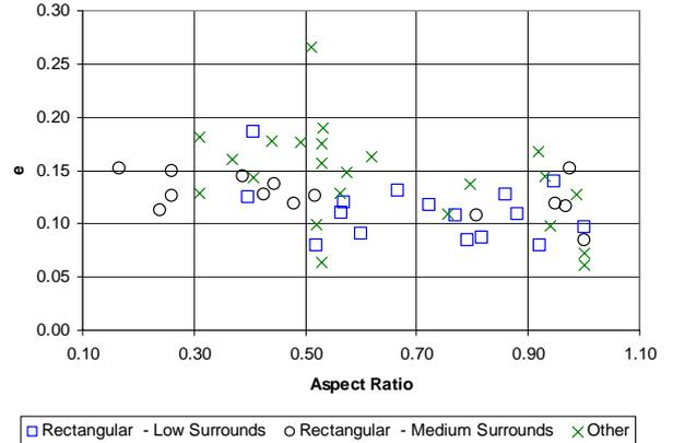
Figure 6. Eccentricity factor based on peak torsional moment and the maximum peak force for the three building groups using the maximum plan form diagonal length of the building.
