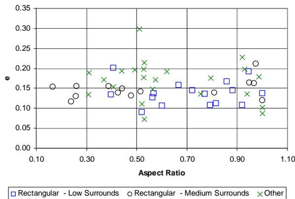
Figure 5. Eccentricity factor based on peak torsional moment and the maximum peak along force for the three building groups.
