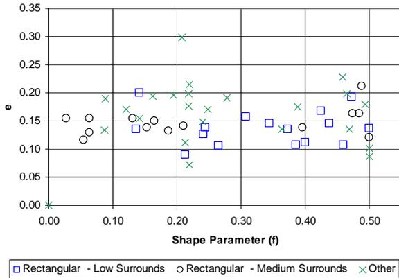
Figure 7. Eccentricity factor based on peak torsional moment and the maximum peak force for the three building groups plotted against the shape parameter  $f$ .
