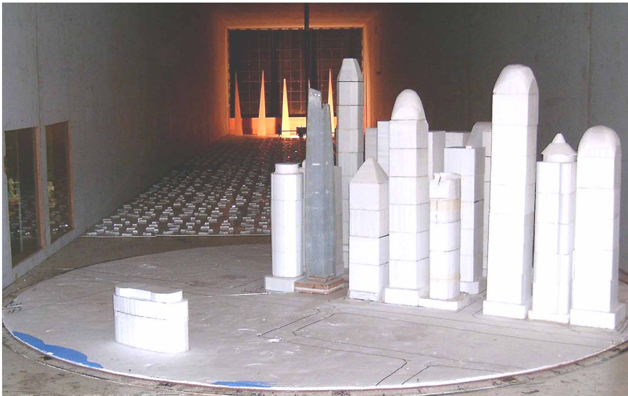
Figure 6: Example of a model set-up at Windtech's wind tunnel facility to determine the design wind pressures for a tall apartment building
