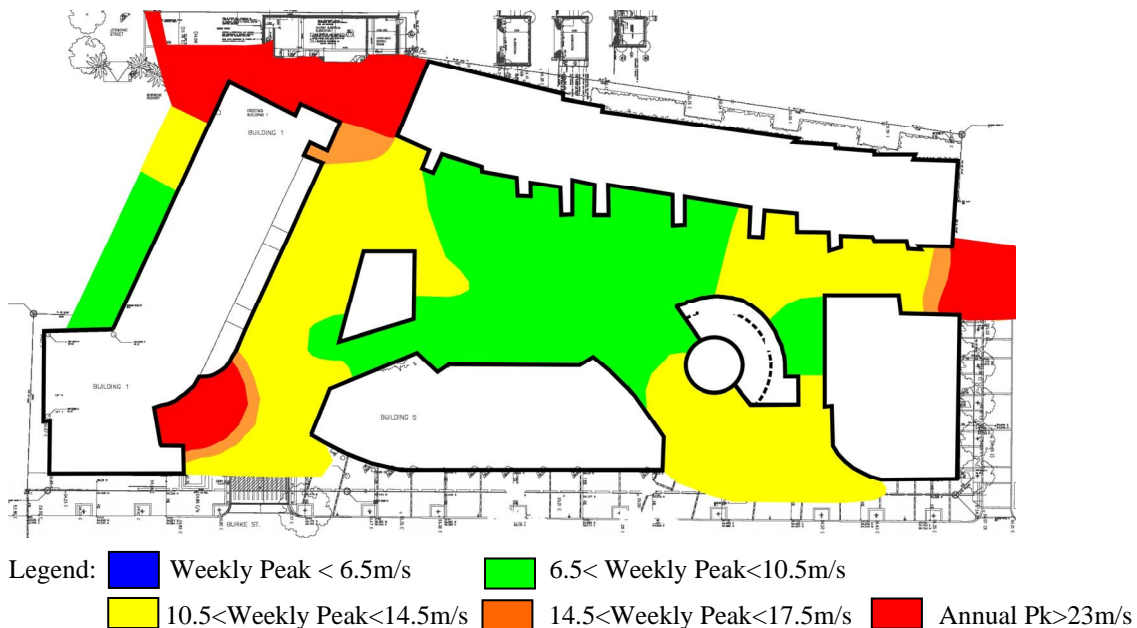
Figure 7: Results based on recommended criteria for weekly maximum Gust (as per Table 1)
